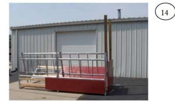
Put on the front wall. Let this go as close to the ground as you wish. If you wish you can leave some clearance from the ground to keep it out off the muck, or you can run it all the way to the ground to keep the muck from running under the feeder.
