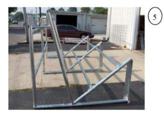
If you are making a long run of this feeder keep an eye open to keep it in a straight line. If the line is fairly straight the feeder will stay square.
