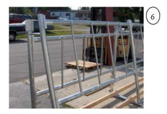
After the main frame is straight put in all the stanchion bars. After this is done it is time to tighten all the bolts. Short ones in the front, long ones in the middle. Now tighten all the bolts.
