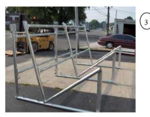
After the BK-3's are bolted into the front then bolt the BK-4's into the middle section. (The BK-4's have four holes in them).
